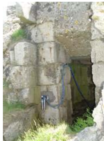
Dual vibrating wire tiltmeters monitor rotations ( \pm 10 arcsecond resolution) in either axis in the machine gun bunker ("tobruk") at the face of the cliff.
