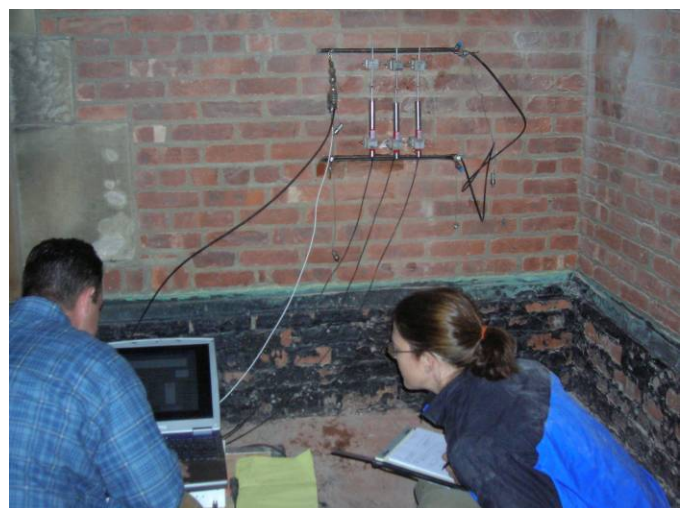
In situ deformability testing
