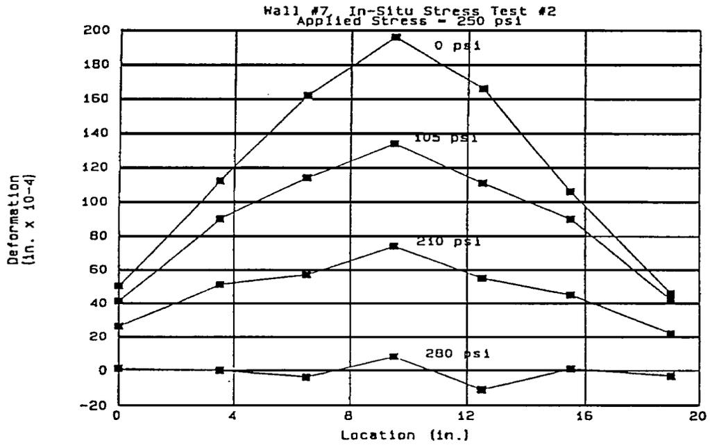
Figure 4. Deformations around flatjack slot during an in-situ stress test.
