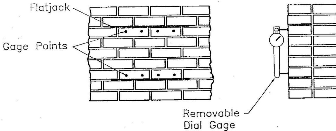
Figure 3. Setup for the in-situ deformability test.
