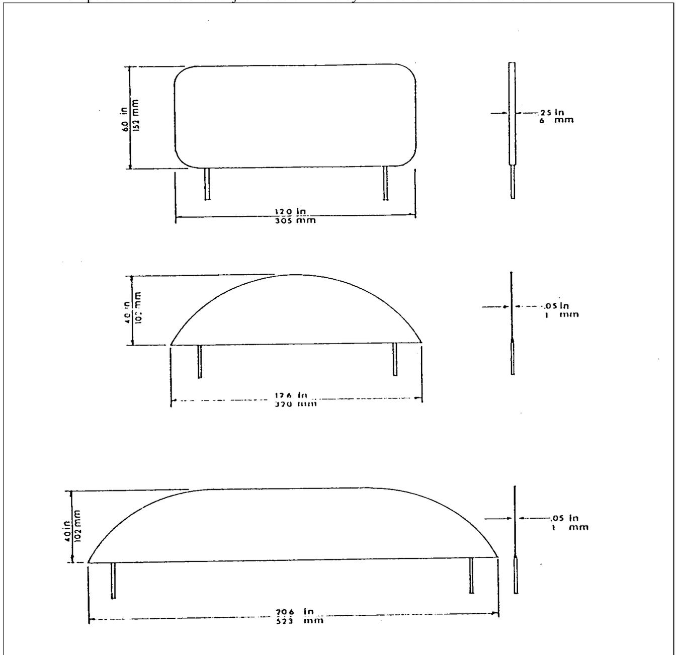
Figure 1. An example of typical flatjack configurations.
