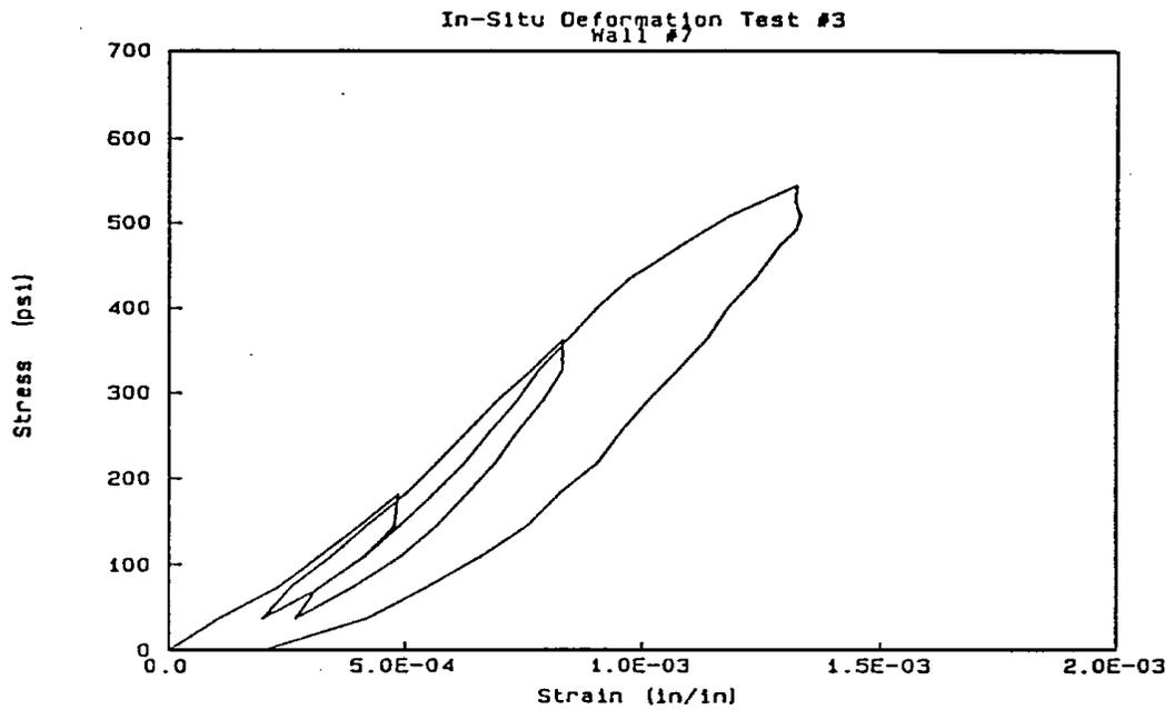
Figure 5. A stress-strain curve obtained during a cyclic in-situ deformability test.
