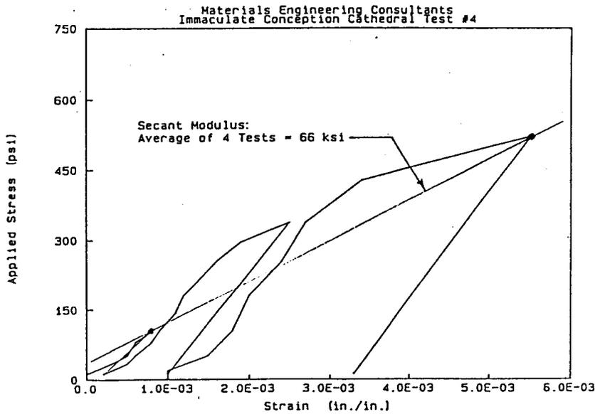
Figure 9. In-situ deformability test conducted on a masonry cathedral in Los Angeles.
