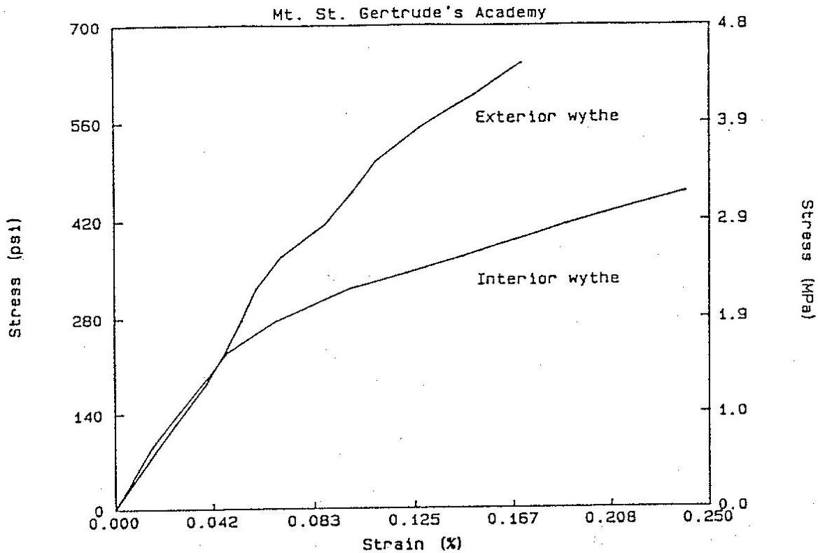
Figure 6. In-situ deformability test results from Mt. St. Gertrude's Academy, Boulder, Colorado. Note the drop in modulus of the load-bearing interior wythe at about 225 psi.
