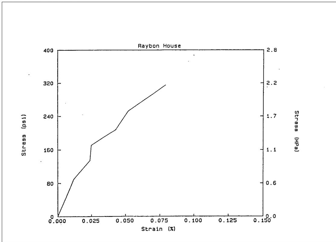
Figure 7. In-situ deformability tests results obtained for the Raybon House, Colonial Williamsburg, Virginia.
