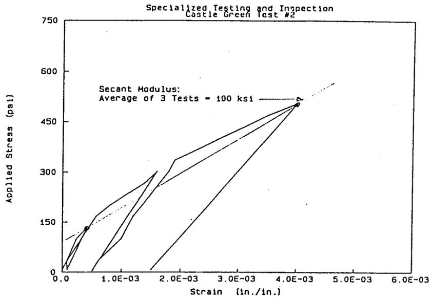
Figure 8. In-situ deformability test conducted on a circa 1900 masonry structure in Pasadena, California.
