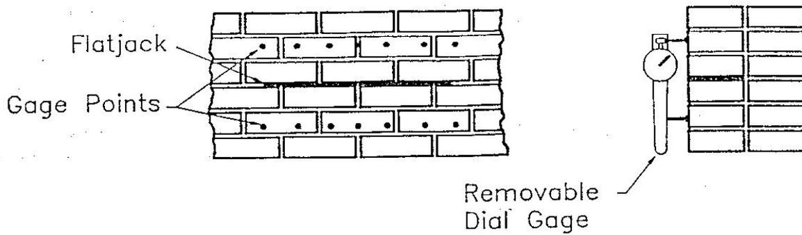
Figure 2. Setup for the in-situ stress test.
